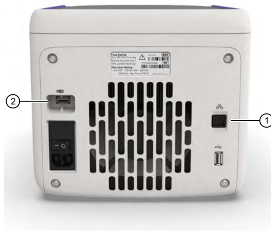
① Ethernet port ② USB port for wi-fi module
